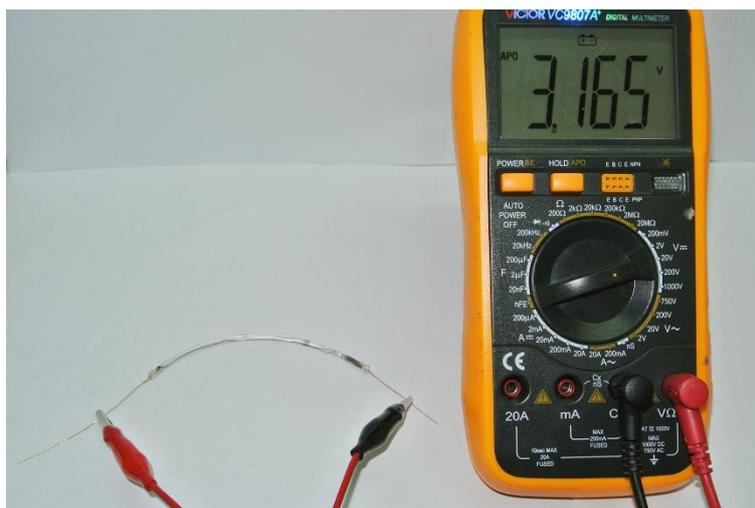
**Figure S20. Open-circuit voltage of a cable-shaped lithium sulphur battery.**
