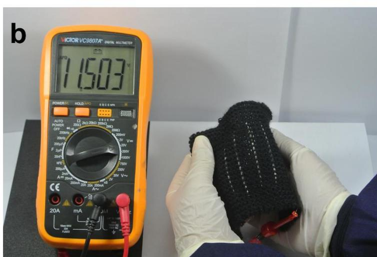
**Figure S22. Photographs of an energy fabric.** The fabric was integrated with 5 cable-shaped lithium sulphur batteries that were serially connected.
